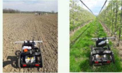
Figure 1. Measurement with a GPR cart and 500 MHz antenna on an empty field (left) and in an orchard (right).
