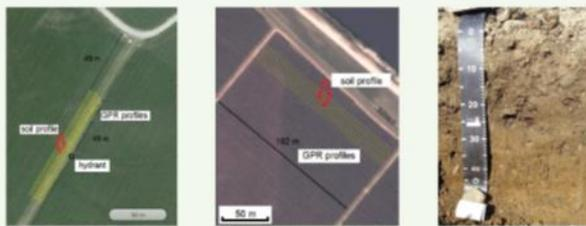
Figure 2. GPR profiles (yellow lines) recorded around the area of soil profiling (red arrows) on an empty field (left) and in an orchard (middle). Soil profile from the empty field is on the right.
