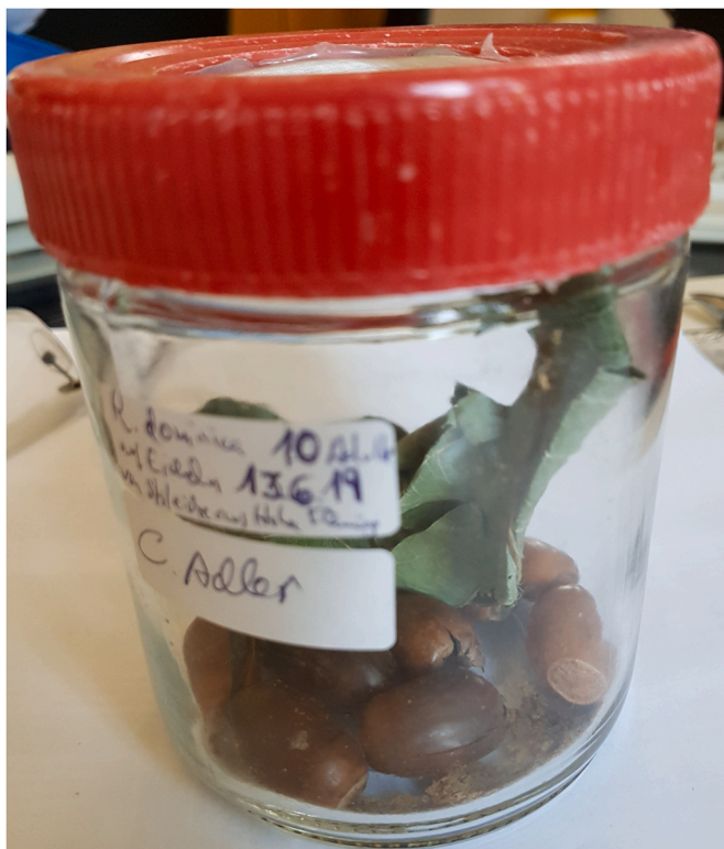
Fig. 3. Jar with 10 adult Rhyzopertha dominica on acorns, three months after starting the test. The dark frass at the bottom depicts insect activity (photo: C. Adler).
